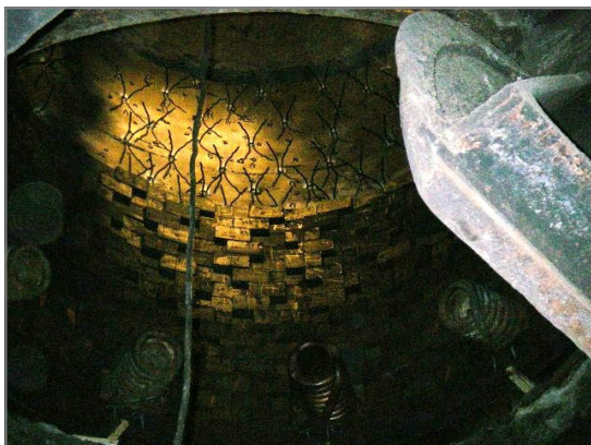
DuraMeltz® - Melt Zone High Conductivity Brick
